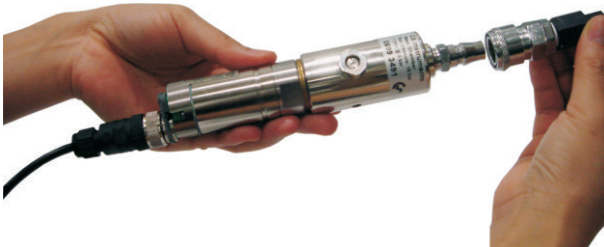
Connection of FA 410 with measuring chamber to compressed air
