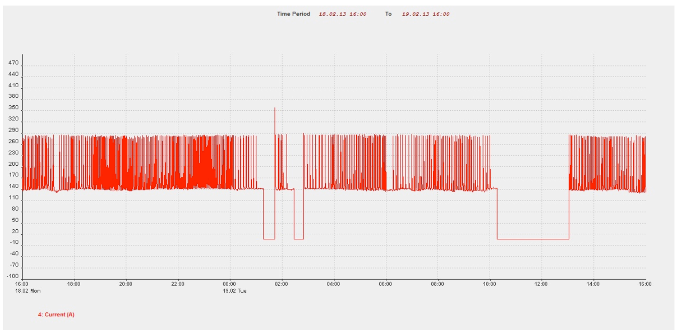
Figure 1: Day profile electrical usage (Compressor 2, Current/Amps) before leak detection
